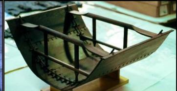
Technological differences between Southerners and Northerners in constructing their ships' hulls do not emerge before the 1st millennium CE. Mortise and tenon was preferred in the South whilst klinker planking won out in the North.
